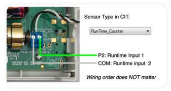
Wiring, TW-140B-R (Manufactured before Q4, 2016)
