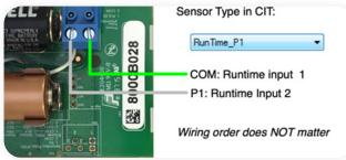
TW-160B-RC, TW-170B-RC & TW-180B-RC dry contact/relay input Runtime version
