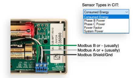
Modbus wiring designation on various meters is unfortunately *not* consistent! Some meters indicate A and B, whereas others might only have + and -. Yet others combine them: A(-) and B(+) and some are A(+) and B(-)! Refere to this table for the currently supported Meters.
